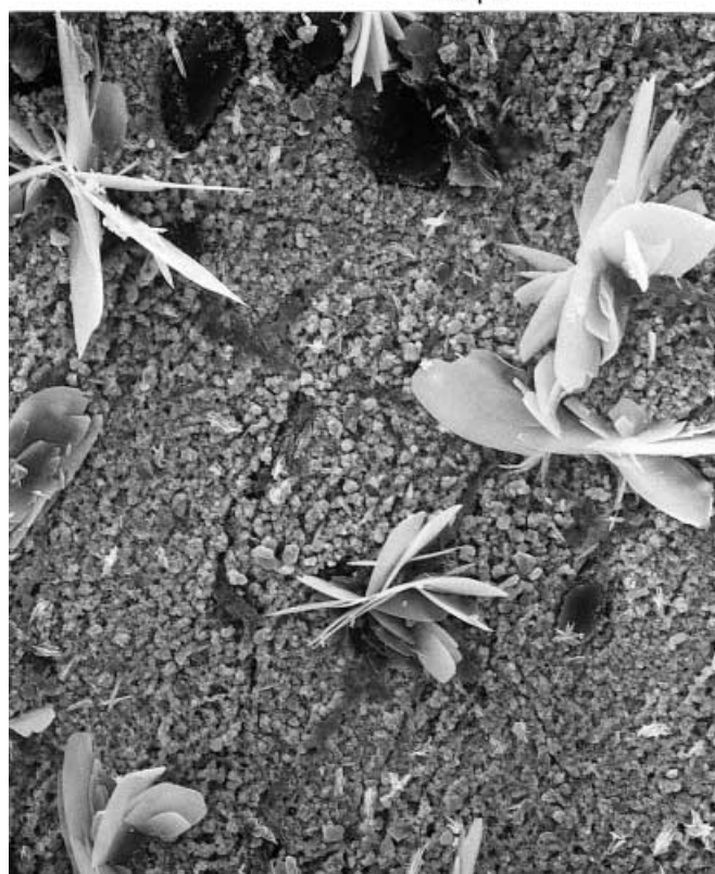
Fig. 3a–c SEM photographs of lead electrode: a after polishing and rinsing; b after ten successive oxidation-reduction cycles in 6 M H 3 PO 4 at 20 °C; c after ten successive oxidation-reduction cycles in 12 M H 3 PO 4 at 20 °C. Experiments were started at –0.7 V and stopped after the last reduction scan at –0.7 V
